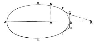
it so that the tangents GF and HI make the angles FGB and IHB each equal to 135°, then the solid generated by the revolution of the figure ADFGBHIE about AB will encounter less resistance than the original solid.
