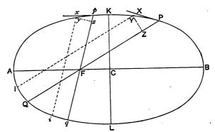
intervalls once in the beginning of every physical moment; and let the first action be upon the body in P, the next upon it in Y, and so on perpetually; so that the body may move from P to Y in the chord of the arch PY, and from Y to its next place in the ellipsis in the chord of the next arch, and so on for ever.
