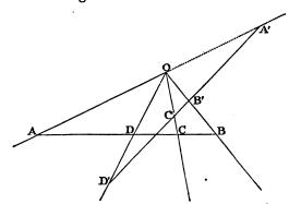
Suppose OA, OB, OC, OD to be a pencil, and let a transversal A'B'C'D' meet three straight lines of the pencil, and the fourth AO produced at A'. The angles A'OB', AOB are supplemental; and so are AOD, A'OD'; and so on. Hence any anharmonic ratio formed on ABCD is equal to the corresponding ratio formed on A'B'C'D'.
