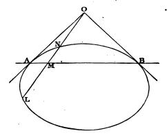
with AB form an harmonic pencil. A particular case is that in which the point in AB is the intersection of the tangents at N and L, which we know will meet on AB produced. (See Arts. 103, 185.)
